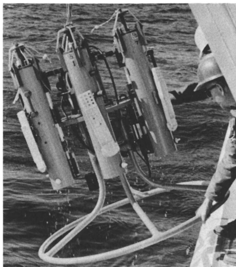
Figure 3. Rosette sampler with 10-l. top drop bottles
